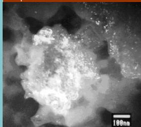
Fig.7 a,b TEM image and diffraction pattern (SEAD) of amorphous phase found in the magnetically treated samples.
