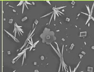
Fig.2 With the application of 1.2 T magnetic fields the main crystal forms are aragonite and vaterite. (Magnification 200 X)
