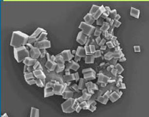
Fig. 1. SEM images of the precipitated particles. Without magnetic field the formation of calcite (trigonal structure) is predominant. (Magnification 200 X)
