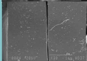
Fig. 8. SEM image of the inner surface of the Si tube used for the experiment
