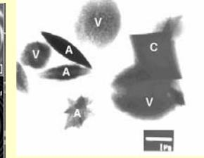
Fig.6 TEM image of various crystals obtained in treated samples: C - calcite, A - aragonite, V - vaterite
