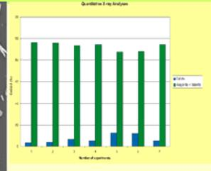
Quantitative X-ray analyses of seven experiments under the same experimental conditions showing the enhanced ratio of aragonite+vaterite to calcite, in the presence of magnetic field.
