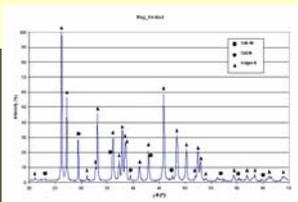
The diffraction spectrum of precipitated CaCO3 obtained from water treated with the applied magnetic field.
