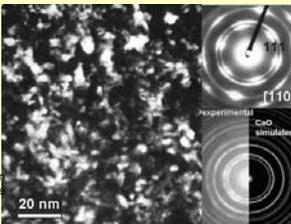
Fig.5 Dark-field TEM image of decomposed vaterite. Insets (upper): SAED patterns of textured CaO in [110] zone axis. Circles (arcs) indicate randomly oriented nanocrystals of CaO. Lower inset: comparison of experimental and simulated SAED patterns for cubic (Fm-3m) CaO
