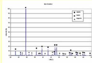
The diffraction spectrum of precipitated CaCO3 obtained from non-treated water.
