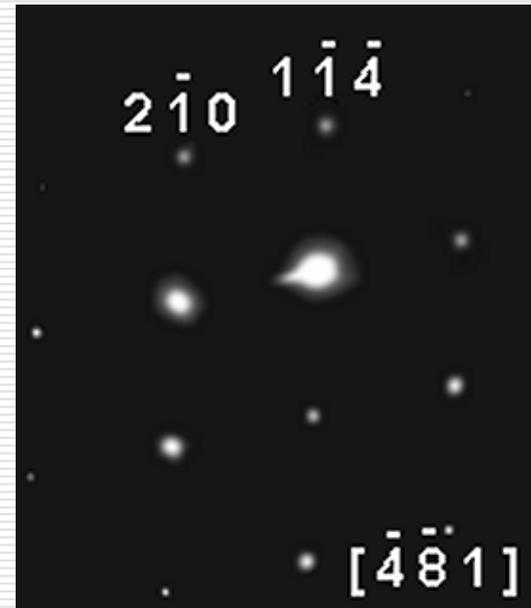
*(A) TEM image. (B) diffraction pattern (SAED). → Calcite*
