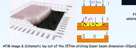
AFM image & Schematic lay out of the 157nm etching (laser beam dimension >20µm).
