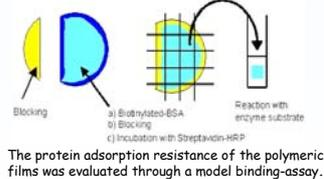
The protein adsorption resistance of the polymeric films was evaluated through a model binding-assay.
