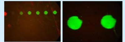
Microarrays consisted of two proteins, rabbit IgG (green) and B-BSA (red), deposited successively after ablation of PTFEMA film and creation of approximately 400µm spots. Spots were visualized after reaction with anti-rabbit IgG antibody labeled with Alexa Fluor 488 (green) and streptavidin labeled with Alexa Fluor 546 (red)
