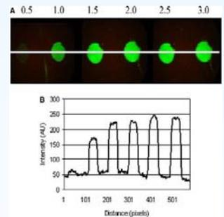
Fluorescence image (a) and fluorescence intensity (b) of the spots created on PTFEMA film for ablation times of 0.5, 1.0, 1.5, 2.0, 2.5, & 3.0 min, respectively. Spot diameter is approximately 400μm
