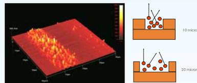
AFM image of irradiated area where stacking of dissociated products on the surface of the polymer is indicated. When the laser beam was ~10µm, the dissociated products were stuck on the polymer surface forming pillars due to enhanced collision rate. The nano/micro-size of the pillars is increasing under prolonged irradiation.
