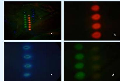
Fluorescence detection of three proteins deposited on laser ablated spots. Spotted-microarray consisted of three (a) one (b), (c) & two protein (d) respectively.
