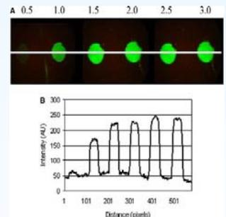
Fluorescence image (a) and fluorescence intensity (b) of the spots created on PTFEMA film for ablation times of 0.5, 1.0, 1.5, 2.0, 2.5, & 3.0 min, respectively. Spot diameter is approximately 400µm
