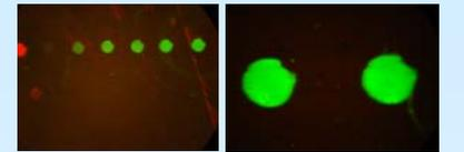
Microarrays consisted of two proteins, rabbit IgG (green) and B-BSA (red), deposited successively after ablation of PTFEMA film and creation of approximately 400μm spots. Spots were visualized after reaction with anti-rabbit IgG antibody labeled with Alexa Fluor 488 (green) and streptavidin labeled with Alexa Fluor 546 (red)
