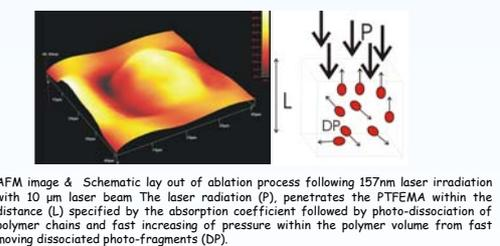
AFM image & Schematic layout of ablation process following 157nm laser irradiation with 10 μm laser beam. The laser radiation (P), penetrates the PTFEMA within the distance (L) specified by the absorption coefficient followed by photo-dissociation of polymer chains and fast increasing of pressure within the polymer volume from fast moving dissociated photo-fragments (DP).
