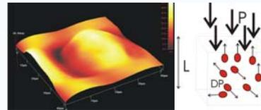
AFM image & Schematic lay out of ablation process following 157nm laser irradiation with 10 µm laser beam. The laser radiation (P), penetrates the PTFEMA within the distance (L) specified by the absorption coefficient followed by photo-dissociation of polymer chains and fast increasing of pressure within the polymer volume from fast moving dissociated photo-fragments (DP).
